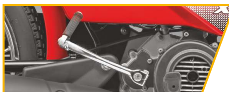
KICKER ON THE RIGHT SIDE
