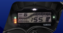
MULTI-FUNCTION LCD INSTRUMENT CLUSTER WITH GEAR SHIFT INDICATOR
