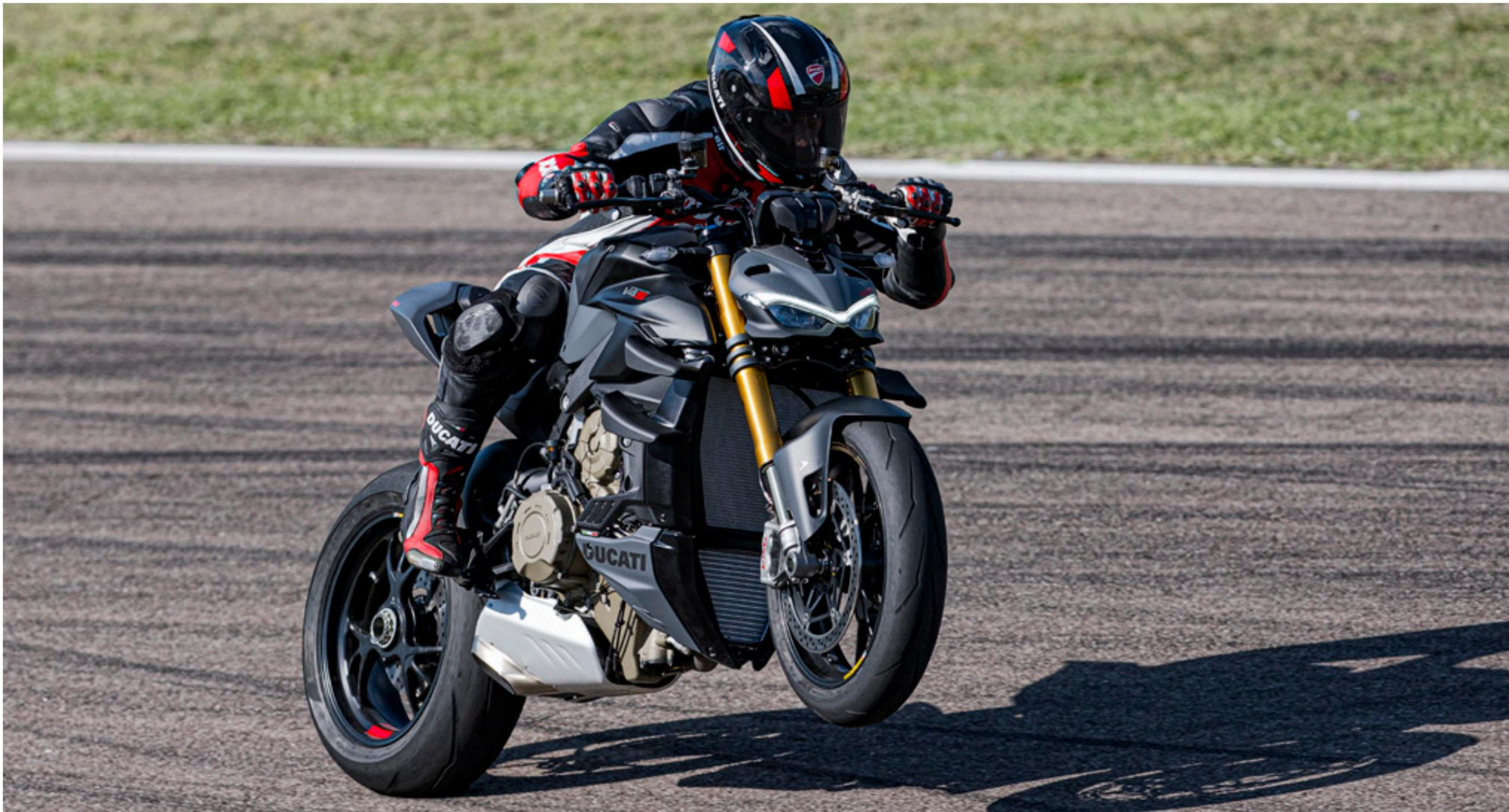
when entering a curve for a spectacular and safe ride. Level 1, not associated by default to any of the Riding Modes, is recommended for experienced riders in track use. It guarantees a racing intervention of the ABS system which acts only on the front wheel. Both the “cornering” function and the anti-lift up intervention are disabled to generate maximum performance.
