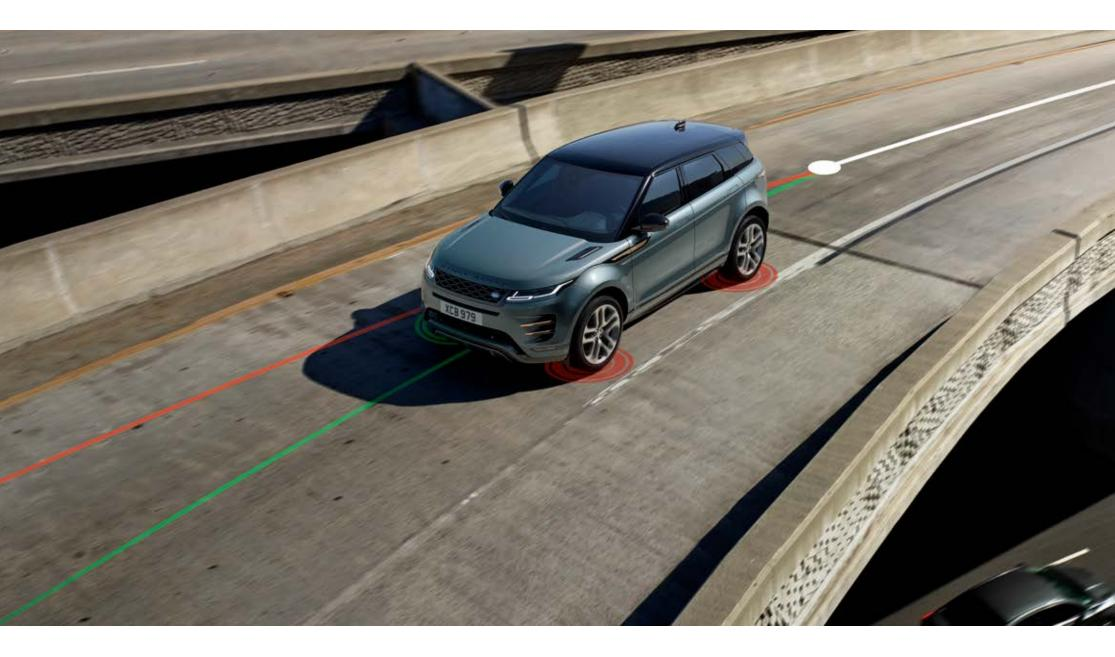
— UNDERSTEER DETECTED — FULL TORQUE TO OUTER WHEELS
