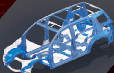
High Tensile Steel Body Construction with Tailor-welded Blanks and Side Anti-intrusion Bars
