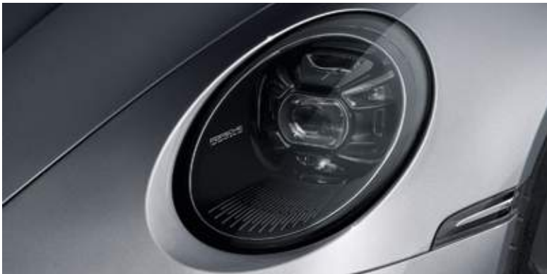
LED main headlights with matrix beam in black including Porsche Dynamic Light System Plus (PDLS Plus)
